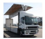
The other popular source of movement is a wing van truck. It's a large scale truck that opens from the side, making it easy to load and unload compared to a container where the doors are on the edges. The downside is that even the largest wing van trucks are not a full size 40ft container. So they're maneuverable but small.
