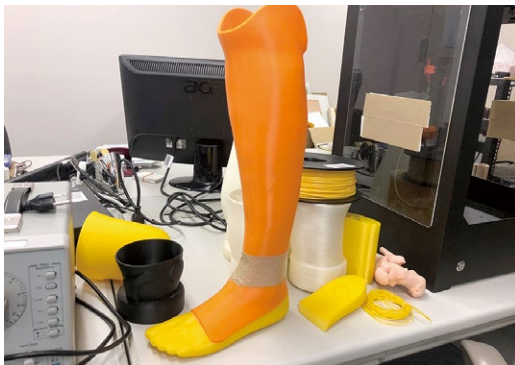
A 3D-printed prosthetic leg prototype and 3D printer (right).
